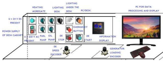
Fig. 8. Control desk for Diesel engine test stand.
